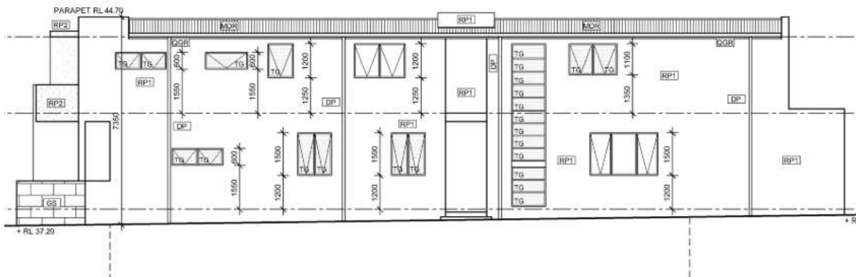
Figure 14. East elevation of the proposed dwelling house (source: N Lyckeno Architect, dated May 2020)
