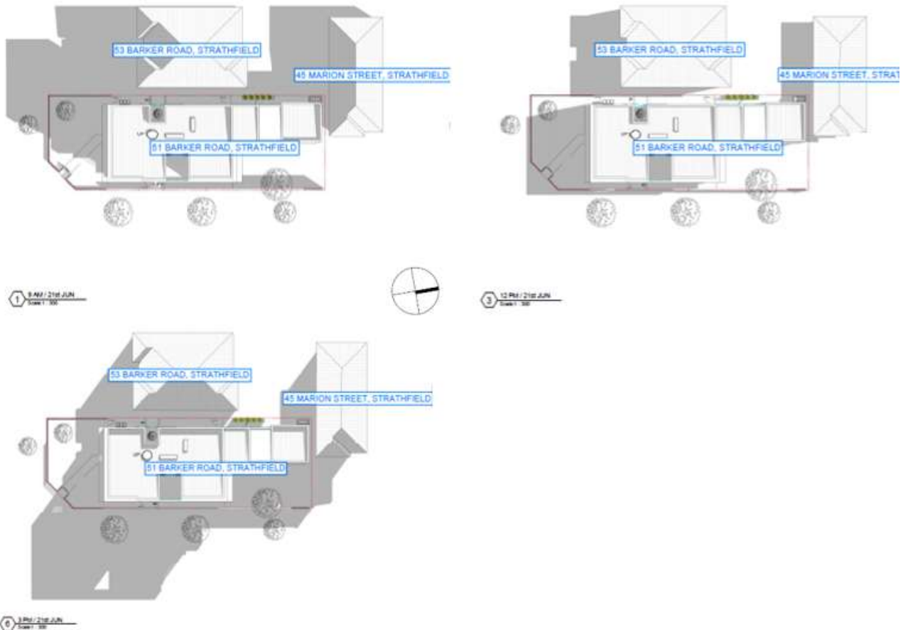
Figure 11: Shadow diagrams of the proposed development and adjoining properties at the winter solstice.
