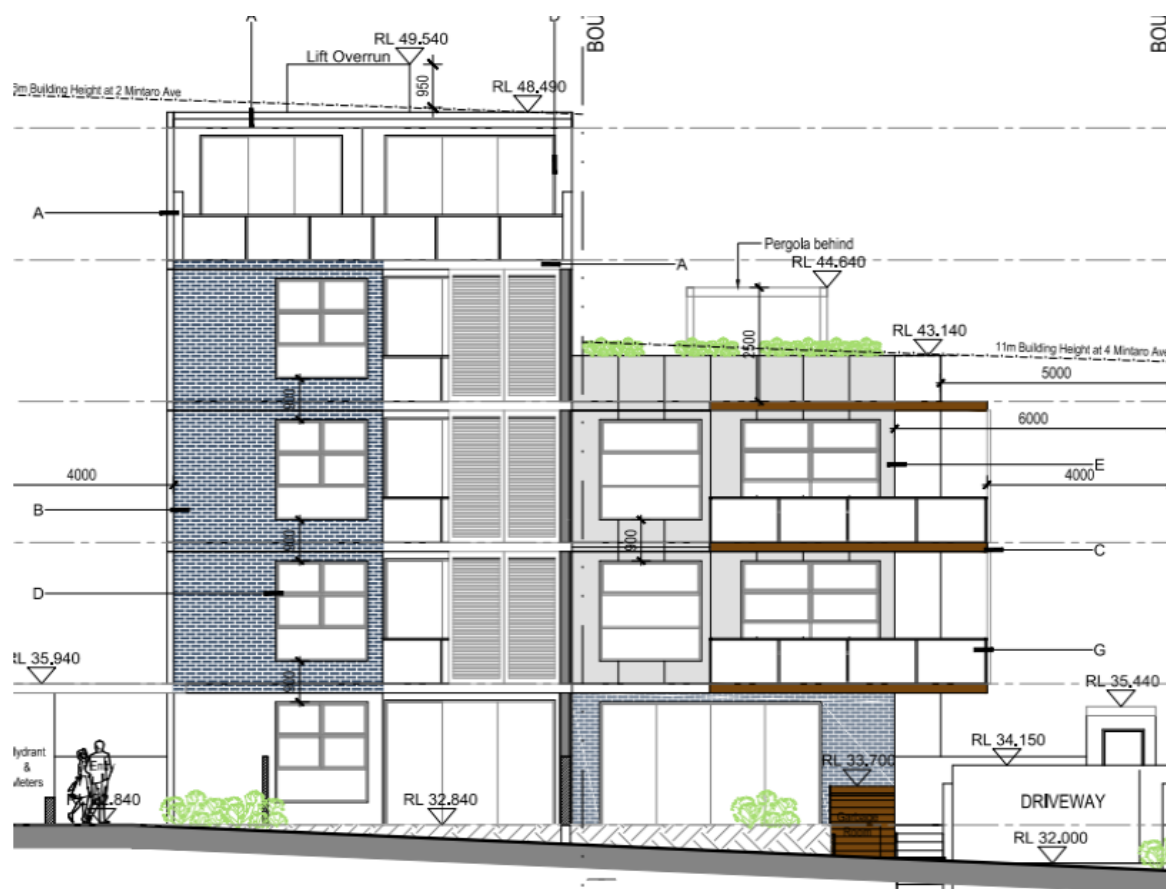
Figure 2: Streetscape elevation of the proposed development.
