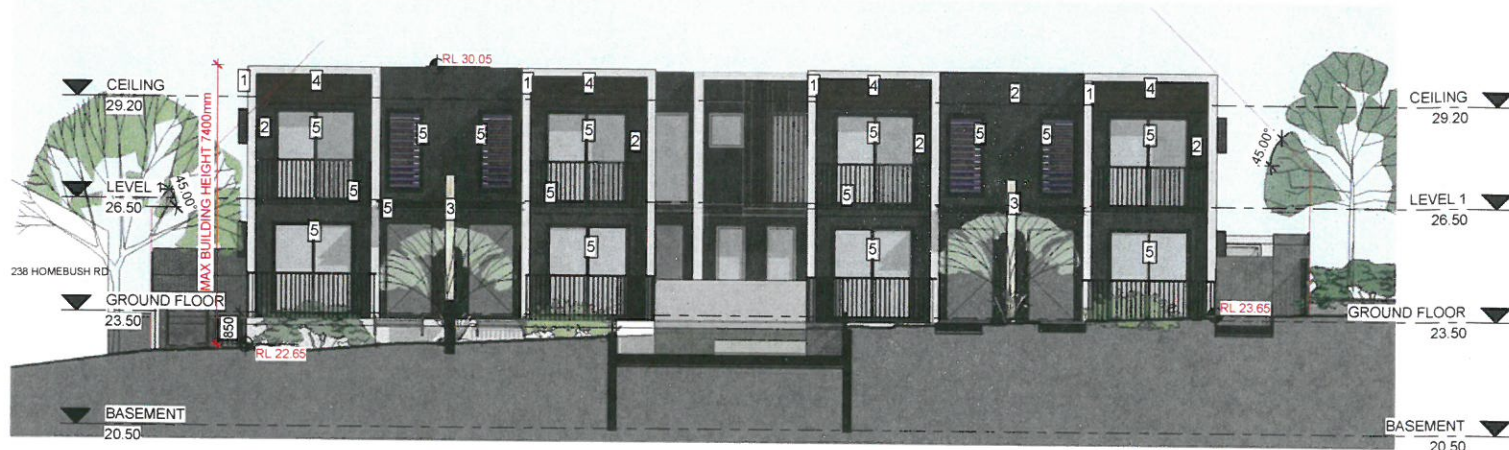
1 WEST ELEVATION (HOMEBUSH RD) A1 1 : 100/A3 1:200
