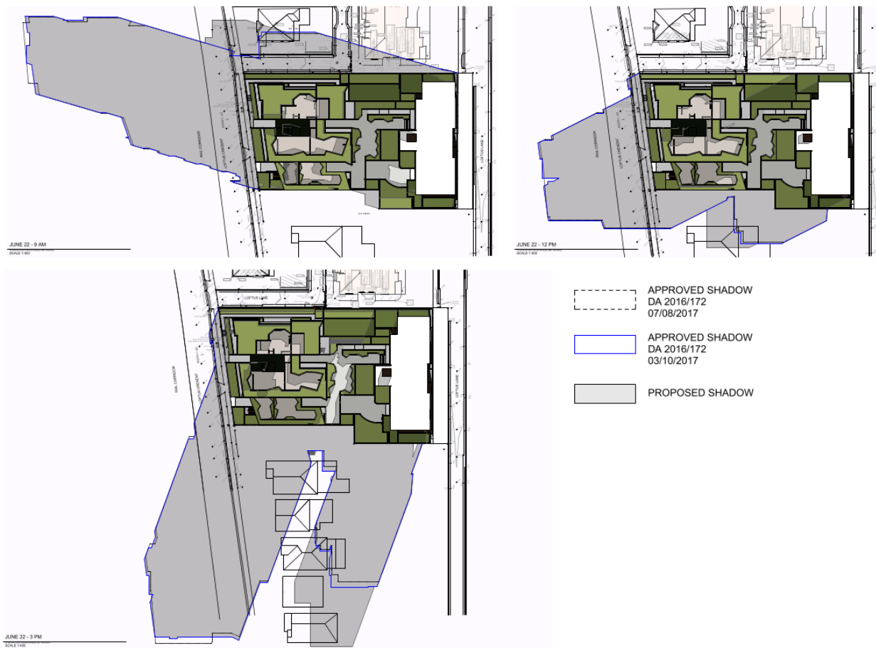
Figure 2: Shadow diagrams of the development as approved and as proposed to be modified.
