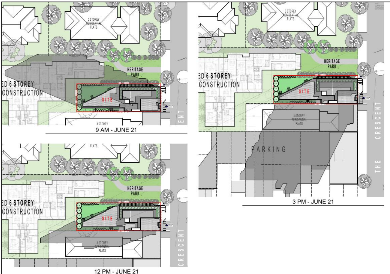
Figure 10: Shadow diagrams of the proposed development.
