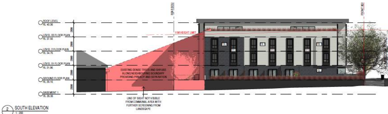
Figure 9. Original Southern elevation showing a part four (4) storey presentation and contravention of the 11m building height control.
